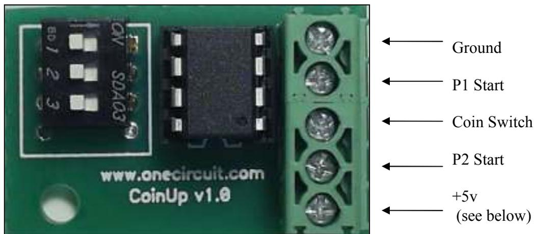
The easiest way to attach the device is to simply use the terminal block to connect it to the existing P1, P2 and coin switch terminals. Unlike the previous version of the CoinUp, the 1UP version does not require cutting into the harness for installation.\*
